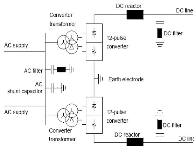
**Figure 2: Main Elements of a HVDC Converter Station with One Bipole Consisting of Two 12-Pulse Converter Unit**
