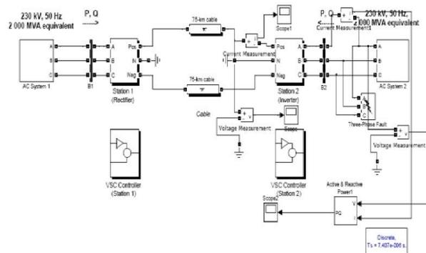
**Figure 7: Main Circuit of Proposed System**
