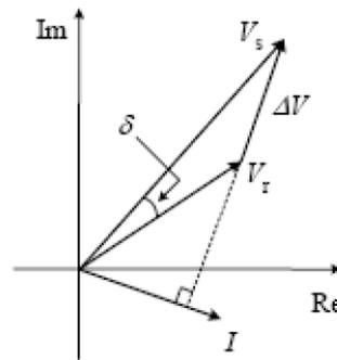
**Figure 3: Vector Diagram of Power Transmission Based on Two AC Voltage Sources Interconnected through a Lossless Reactor**
