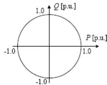
**Figure 4: Active-Reactive (PQ) Locus Diagram of VSC-Based Power Transmission System**
